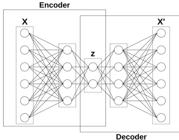
Fig. 1: An Autoencoder with three fully-connected hidden layers.  $X$  is the input layer,  $X'$  the output layer, which is the approximate reconstruction of  $X$ . The output of the second hidden layer is the latent representation  $z$ .
